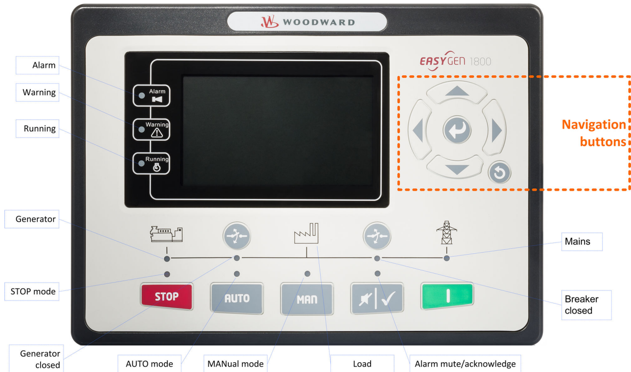
Fig. 8: HMI (front panel) easYgen-1800
