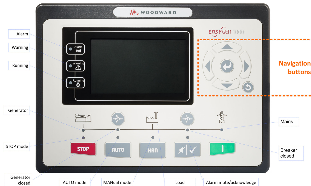
Fig. 32: HMI (front panel) easYgen-1800
