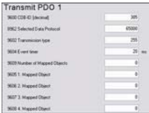
Fig. 205: TPDO configuration for IKD 1 (example ToolKit)
