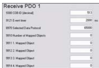
Fig. 207: RPDO configuration for IKD 1 (example ToolKit)
