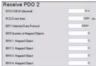
Fig. 215: RPDO configuration for 2nd IKD 1 (example ToolKit)
