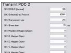
Fig. 213: TPDO configuration for 2nd IKD 1 (example ToolKit)
