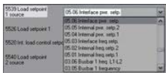
Fig. 268: Setpoint source configuration
