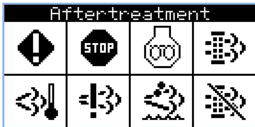
Image 5.28 Example of active Tier 4 Final screen
