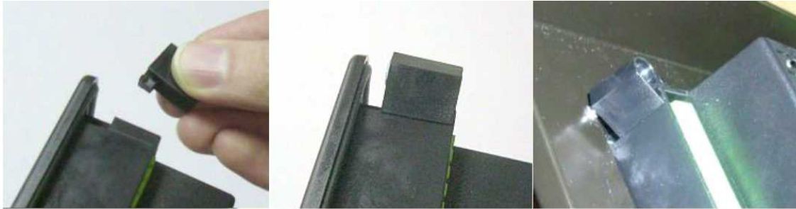
Image 4.2 Connecting the screw holders to the controller and mounted controller on panel door
