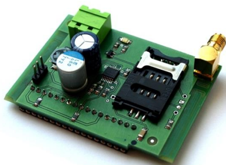
IL-NT GPRS MODULE AND GSM/GPRS SCREEN ON IC-NT DISPLAY
